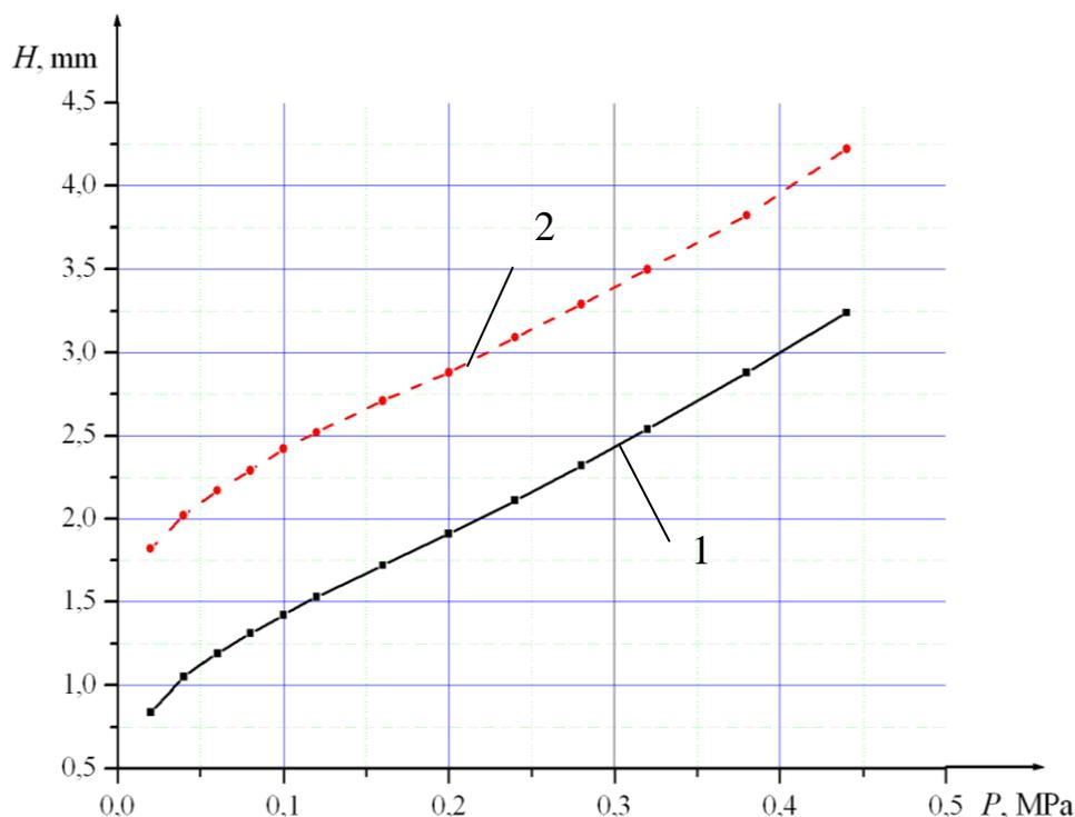
Fig. 4. Dependence «pressure  $p$  - deflection  $H$ » ( the research environment - water);
