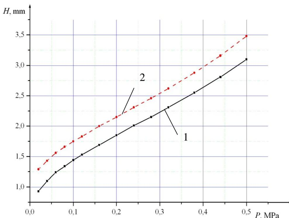
Fig. 5. Dependence «pressure  $p$  - deflection  $H$ » ( the research environment - 10 %-s' solution of hydrochloric acid); 1 - the sample under a magnet, 2 - without a magnet
